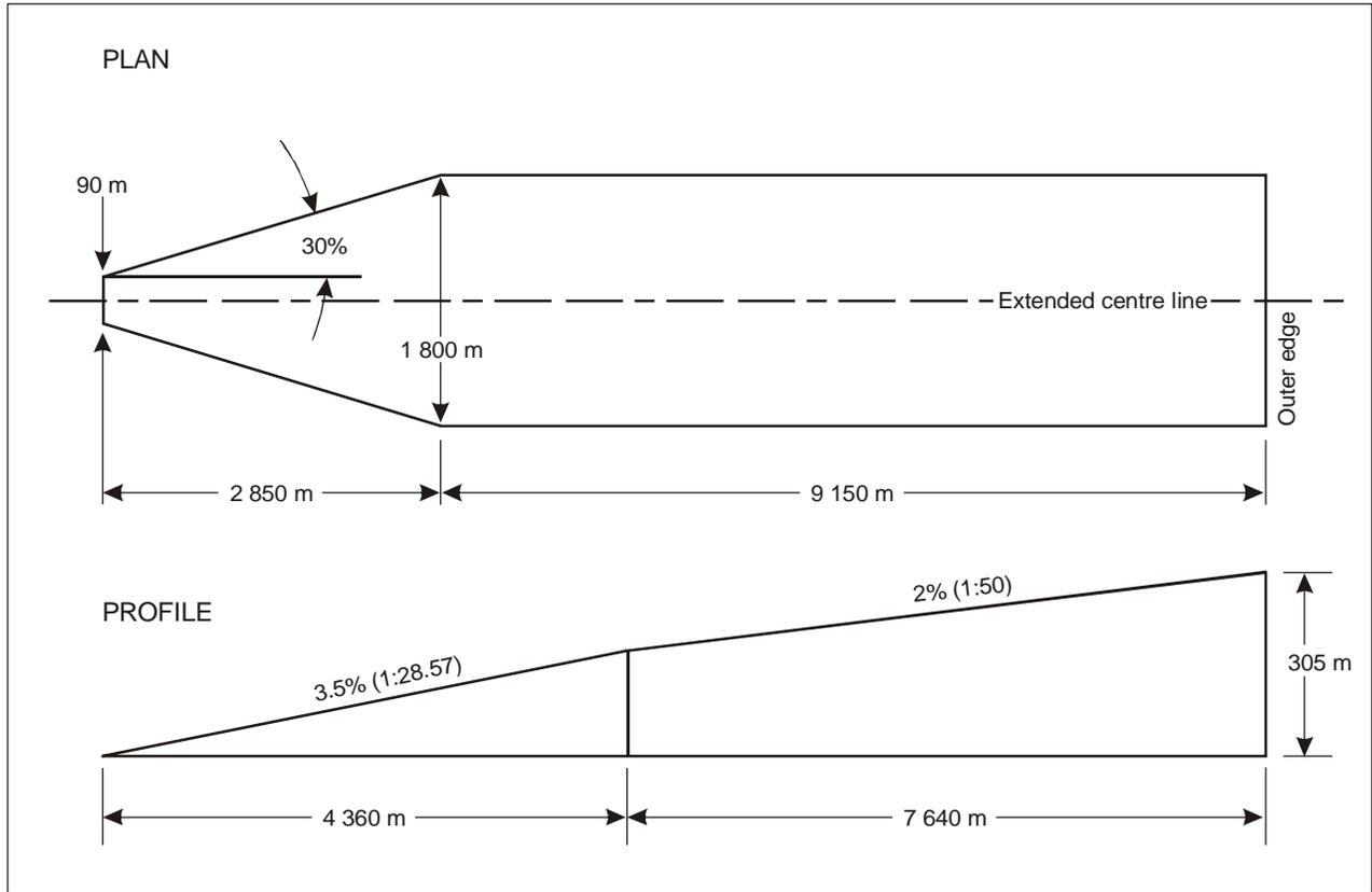
Figure 4-5. Take-off climb surface for instrument FATO
