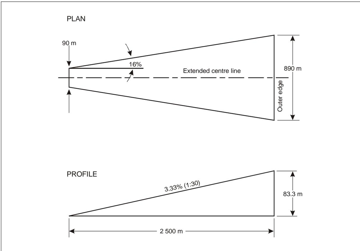
Figure 4-7. Approach surface for non-precision approach FATO
