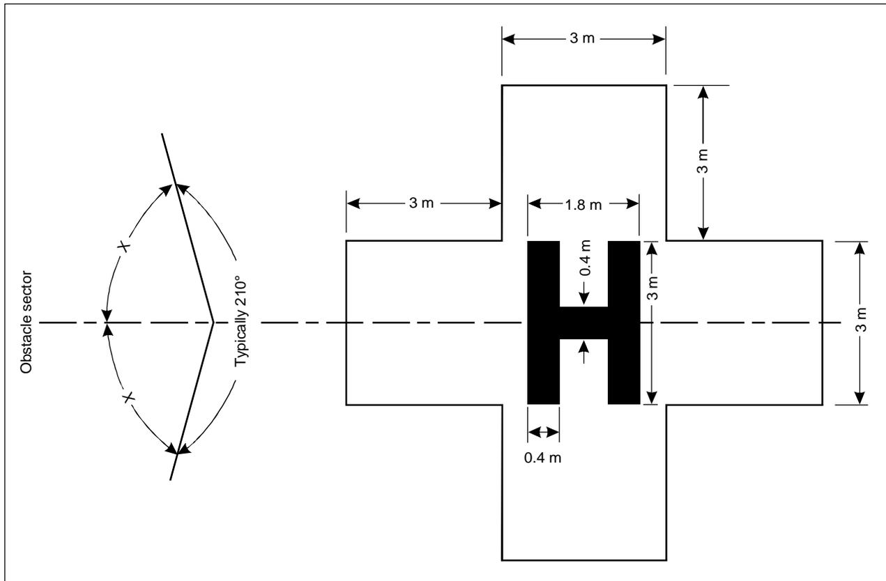
**Figure 5-1. Heliport identification marking**
