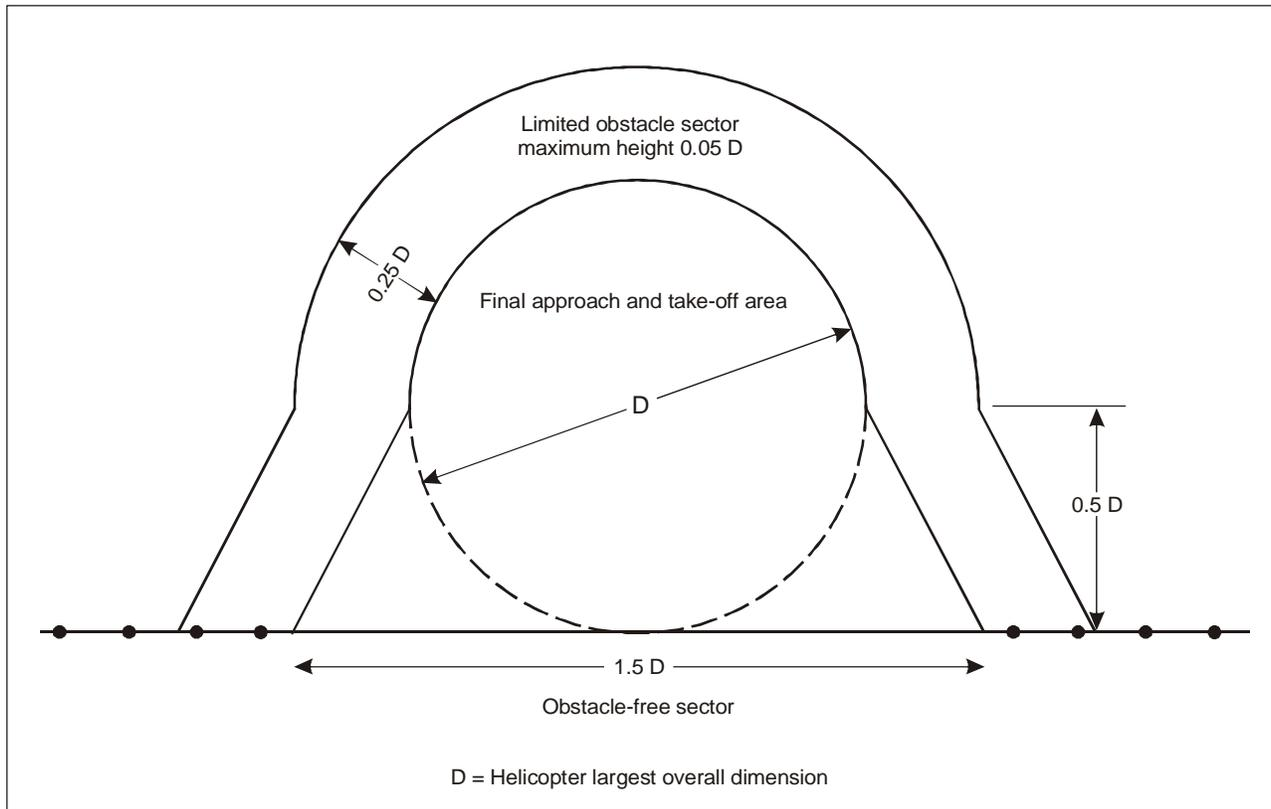
**Figure 4-10. Ship's side non-purpose-built heliport obstacle limitation surfaces**
