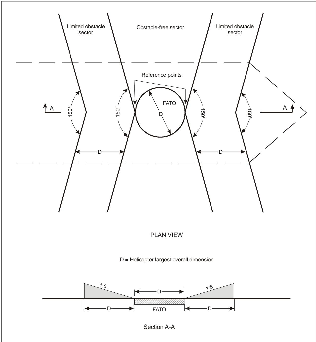
Figure 4-9. Midship non-purpose-built heliport obstacle limitation surfaces
